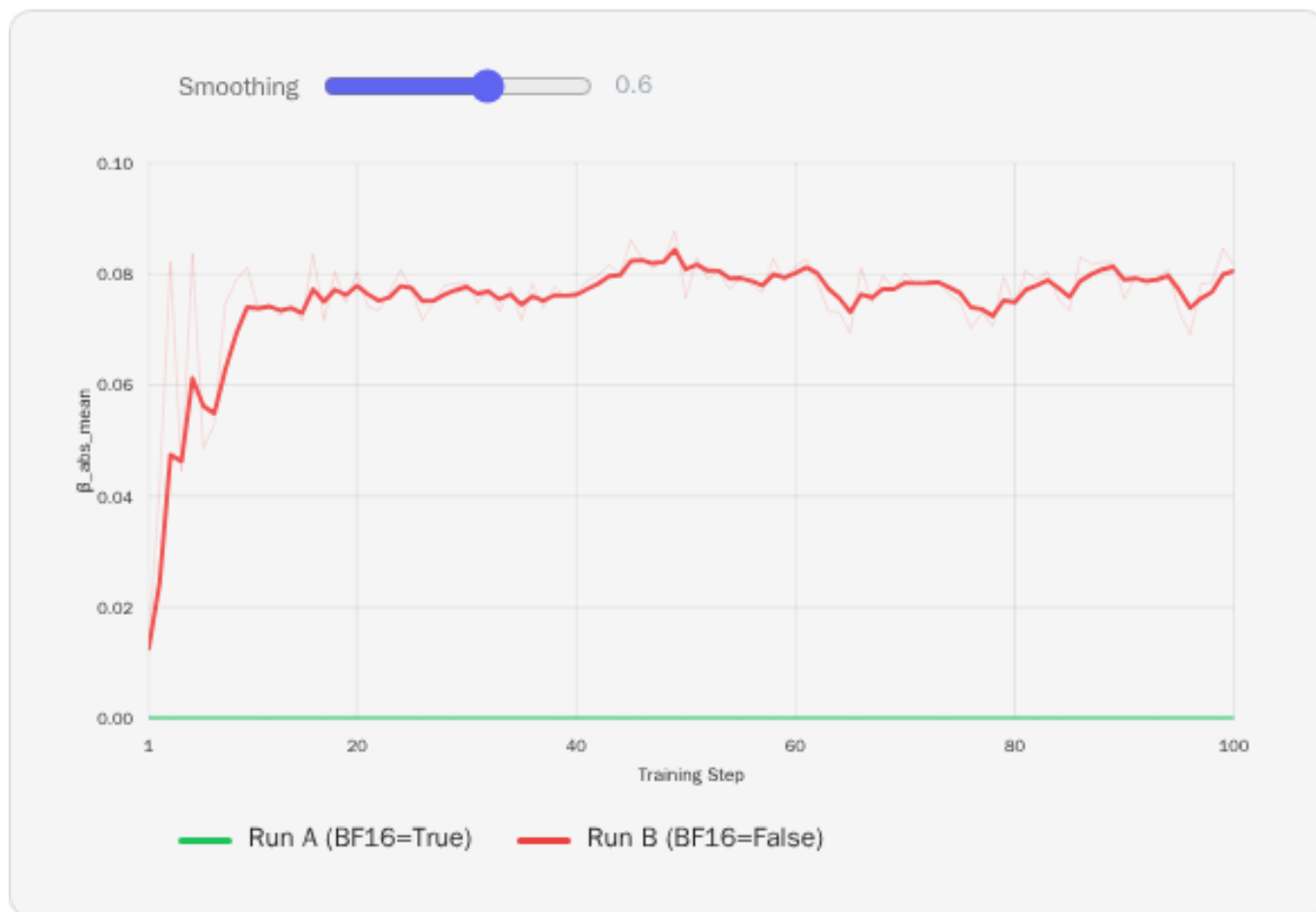
Figure 8 · Mean |\beta| per step. BF16=True produces \beta=0 exactly; BF16=False shows persistent precision gap \sim 0.076
