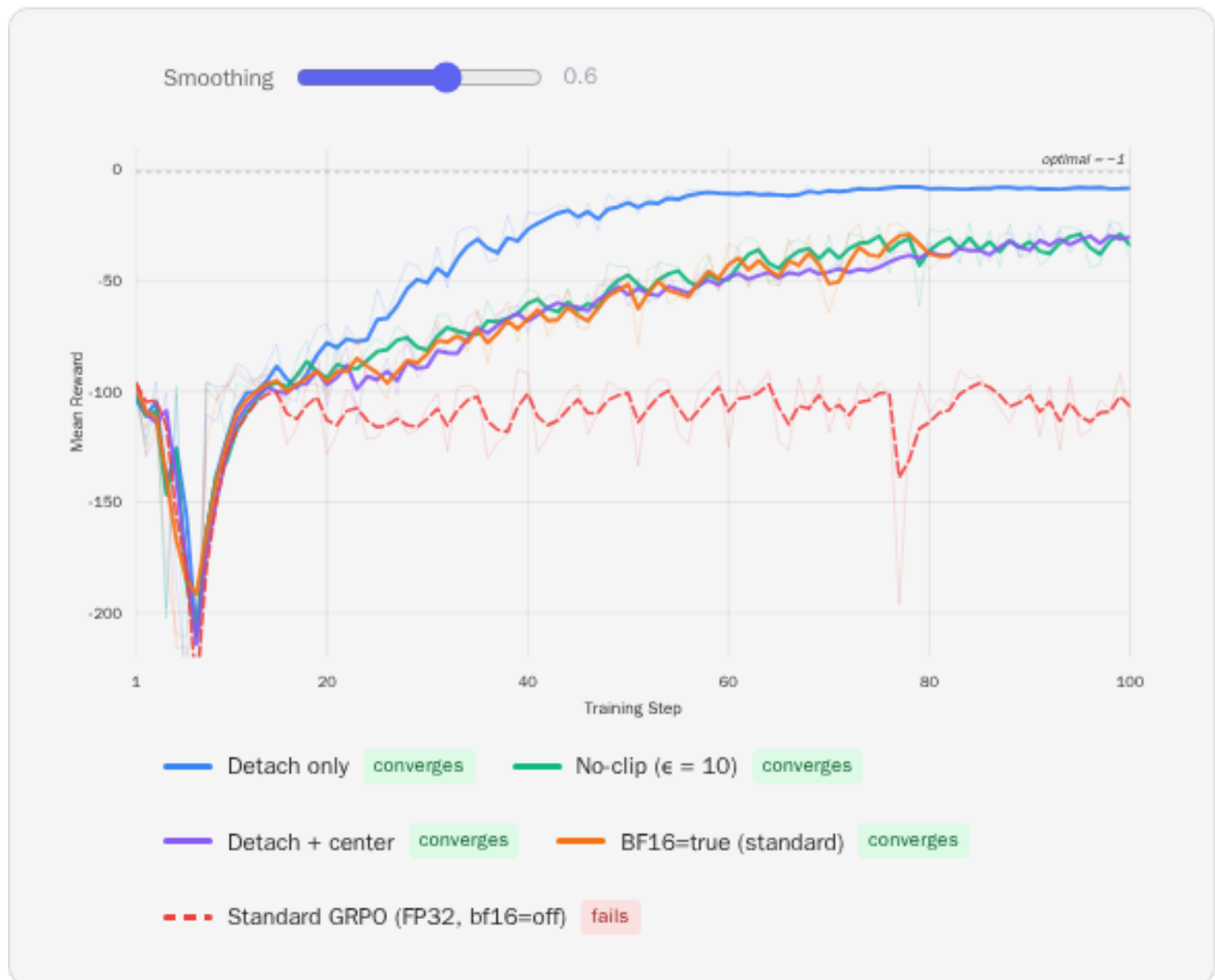
Figure 26 · All three interventions converge. The \epsilon=10 result is decisive: standard PPO with \beta fully intact converges because clipping is disabled.
