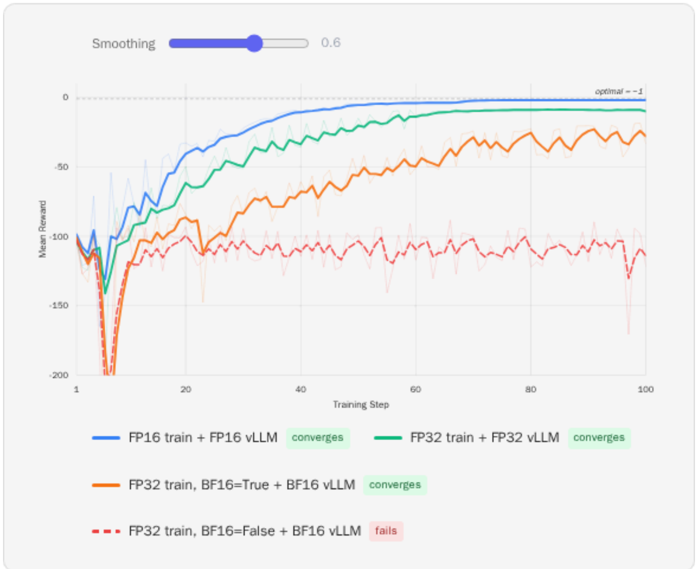
Figure 2 · Mean reward vs training step for four precision configurations. Convergence fails exactly when training and inference use different effective precisions.
